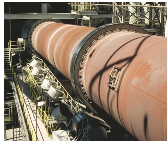
The decomposition of limestone is carried out in a long rotary kiln
